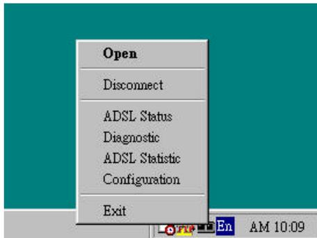
Pointing to the Modem Icon and clicking on the right mouse button will display the Modem Icon options window. From this window, the user will be able to: a) "Disconnect" the modem from or "Connect" the modem to the central office equipment; b) Monitor the ADSL modem status; c) Run a diagnostic test to test the modem; d) Monitor various ADSL statistics and e) configure the PVC values for RFC1577 and RFC1483.
