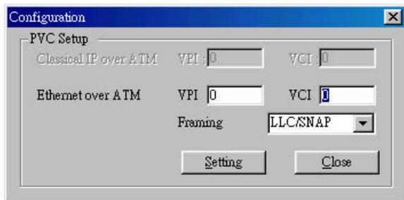
The Configuration menu will allow the user to check or change the ADSL network modems PVC values for RFC1577 and RFC1483. To change the PVC values, simply select one of the RFC protocols, enter the VPI and VCI values, and then click on the Setting button. Click Yes when asked to reboot the system. Click on the Close button to close the configuration window.
