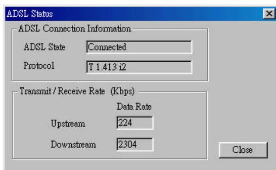
The ADSL Status menu allows the user to monitor the ADSL connection as well as monitor the transmit and receive line rates.
