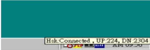
Placing the mouse cursor on the Modem Icon will show a summary of the modems status by displaying the modem's state, upstream line rate and downstream line rate.
