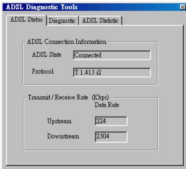
Pointing to the Modem Icon, and clicking on the left mouse button will display the ADSL Diagnostic Tools window. From this window, the user will be able to run Diagnostics, review the ADSL modem status and view the ADSL Statistics. For a more detailed explanation of each window, turn to the appropriate section in this manual for each menu.
